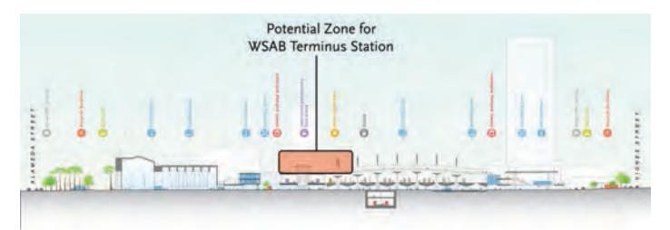
Figure 2-5: Union Station Master Plan cross-section (Gruen + Grimshaw Architects) looking north and showing a potential zone for a new WSAB Terminus Station
