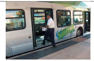
Level Boarding – Similar to rail systems, low floor vehicles and taller station platforms that provide level boarding speeds up the boarding and disembarking processes, especially for wheelchair-bound passengers.
