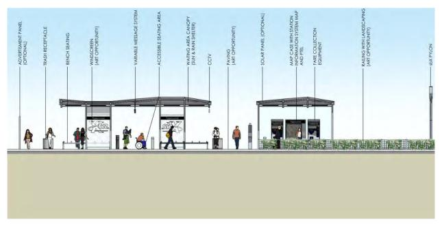
Figure 3-6: BRT Station Components
