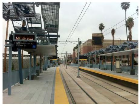
Figure 3-8: Light Rail Station with Overhead Catenary System
