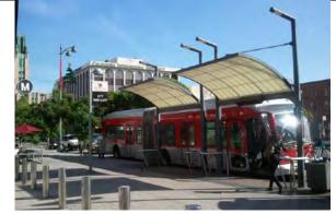
Enhanced Stations (BRT Lite/Rapid Bus) – Metro Rapid service pictured to the left, provide low cost and enhanced stations that include attractive shelters and signage for passengers. These stations reduce vehicle dwell time at stops and promote the identity of the service.
