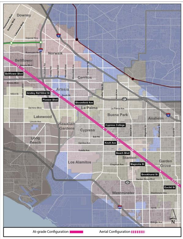
Figure 2.15 – Vertical Configurations on the PEROW/WSAB Corridor
