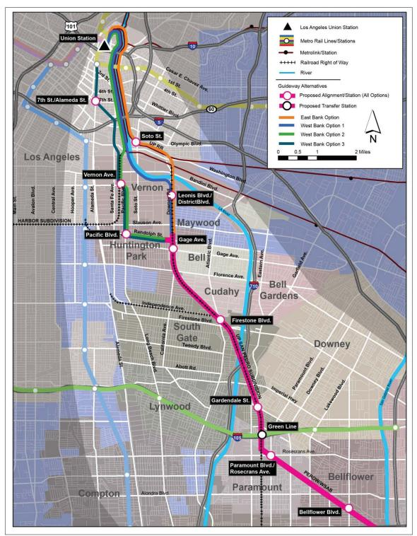
Figure 2.9 – Guideway Alternatives: Northern Connection Area Alignment Alternatives
