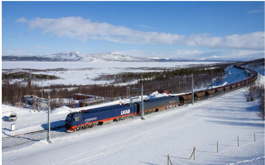
Figure 2.1 Freight Railroad Powered by Electrified Catenary
